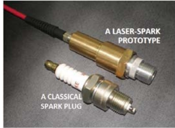
Fig. 1. A laser-spark prototype realized in 2011 in our laboratory.
