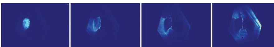
X-ray topographs of potassium alum single crystal
