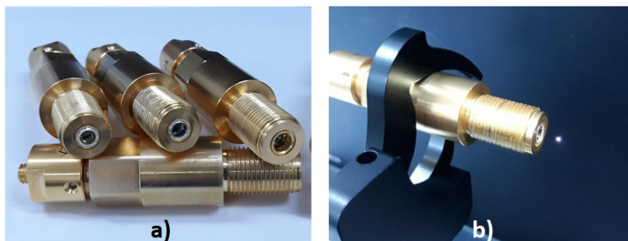
Fig. 4. a) Several “golden” laser spark plugs are shown. b) Air breakdown produced by the 2.80 mJ laser pulse.
