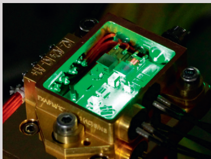
Robust packaged green laser for the Raman experiment of the EXOMARS mission (IOF).
